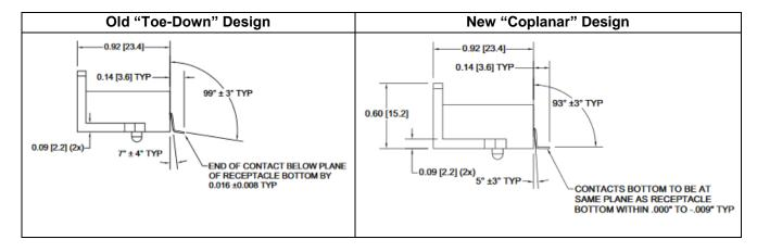
Even though this was a very minor change to the bend angle of the leads, it still constitutes a change in form, so the improved receptacles have new model and part numbers. The table below outlines the replacement "SM" parts for the existing "SMT" parts.
