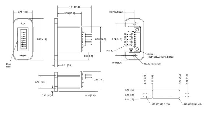
Installation Recommendation: For best water drainage, it is recommended that the receptacle be installed with the output connector above the housing as shown above.
