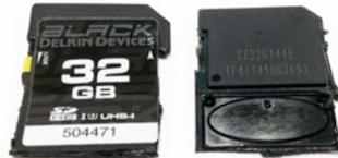
Of the three SD cards tested, the Delkin Black SD card is the only one that claims to be more rugged than a standard SD card. Of the three SD cards tested, the Delkin Black card definitely had the most rugged case. It was by far the hardest to crack open. So why did it require the least amount of force to crack the IC?
