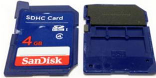
After cracking open the SanDisk SD card, it was apparent that the probe was not positioned over the IC. The video shows that the probe from the force gauge makes a significant depression in the SD card's outer shell before the click is heard.
