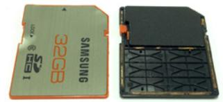
After cracking open the Samsung card, it was clear that its IC was larger than that of the IC in the SanDisk 4 GB card, but it did not even occupy the front half of the card. Based on the video, it appears that the probe from the force gauge was very near or over the bottom edge of the IC.
