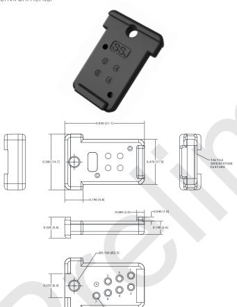
Drawing dimensions are in inches and millimeters [mm]. Dimensions are nominal and subject to manufacturer's tolerances.
