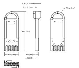
Drawing dimensions are in inches and millimeters [mm]. Dimensions are nominal and subject to manufacturer's tolerances.
